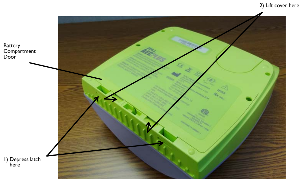
Figure 7: Removing the Battery Compartment Door
